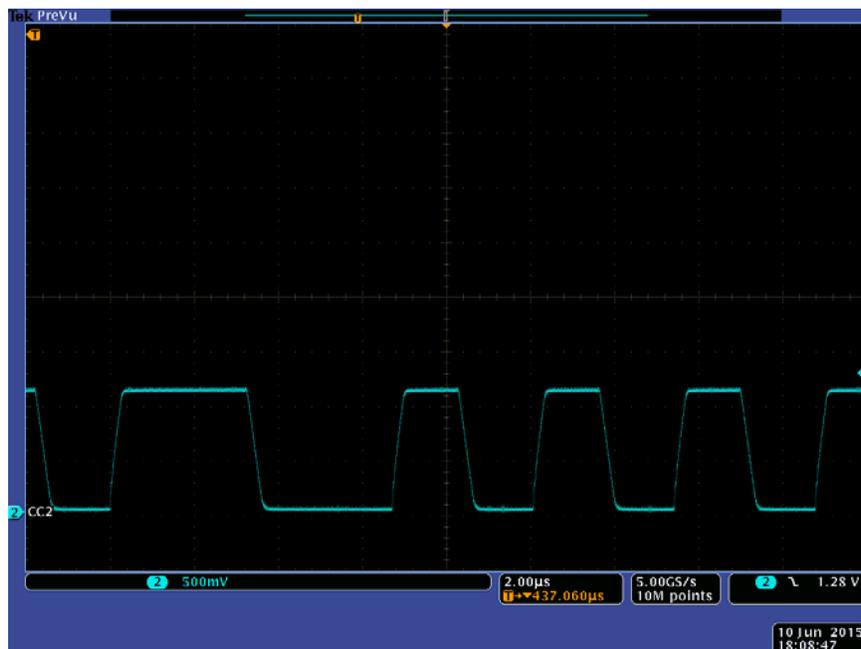
Figure 15. Specification-Compliant PD BMC Waveform
