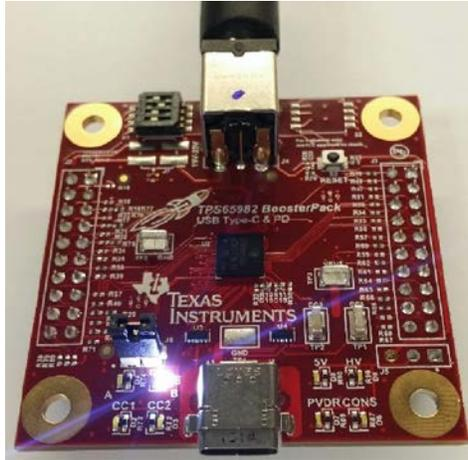
**Figure 2. Powered TPS65982-EVM BoosterPack With Application Firmware**
