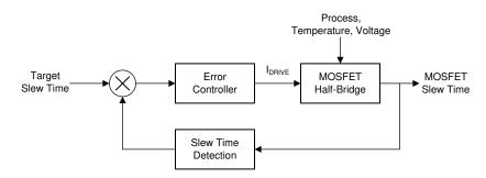
Figure 2-22. Slew Time Control Loop
