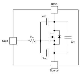
Figure 1-2. MOSFET Circuit Model
