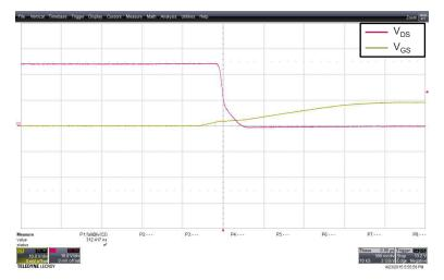
Figure 1-5. Measured MOSFET Slew Rate
