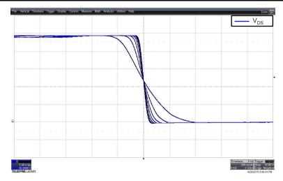
Figure 2-4.  $V_{DS}$  Persistence Plot Across I<sub>DRIVE</sub> Settings
