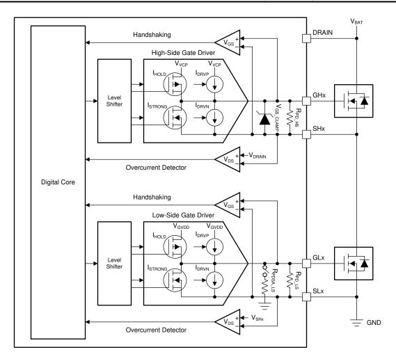
Figure 2-29. Smart Gate Driver Block Diagram
