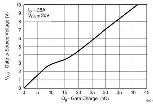
Figure 1-3. MOSFET Gate-Charge Curve
