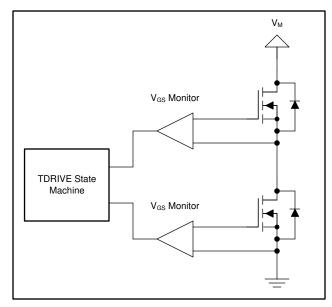
Figure 2-25. V<sub>GS</sub> Monitor Example
