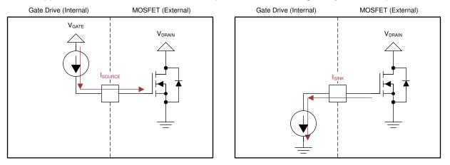
Figure 2-3. Current Source IDRIVE Method
