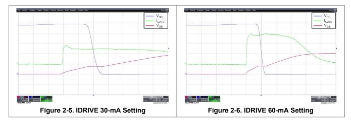
As mentioned in Section 1.4, if a close-to-ideal current source and an accurate MOSFET  $Q_{GD}$  parameter are available, an approximate calculation for the  $V_{DS}$  slew rate can be made. In the table below, the calculated  $V_{DS}$  slew rate is compared to the measured  $V_{DS}$  slew rate for several  $I_{DRIVE}$  settings. In these calculations, assume that the effects of the series gate resistance and additional non-idealities are minimal.
