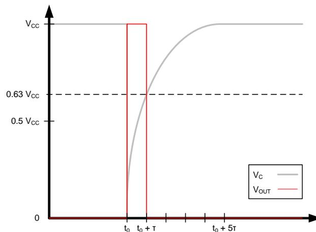
Figure 2. Capacitor Voltage With Aligned Output Pulse (Ideal)
