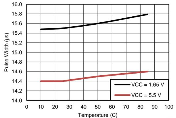
Figure 8. Pulse Width Over Temperature and Supply Voltage Range With C<sub>ext</sub> = 500 pF and R<sub>ext</sub> = 100.7 kΩ
