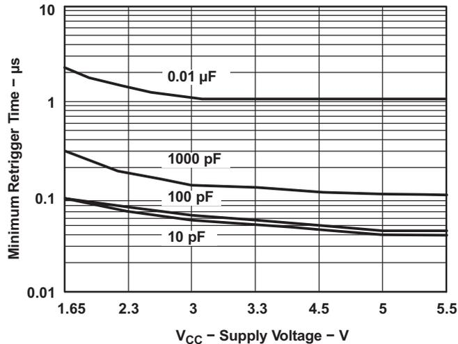
Figure 6. Minimum Retrigger Time vs Supply Voltage
