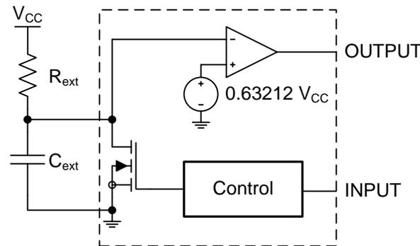
Figure 1. Functional Diagram of a Monostable Multivibrator
