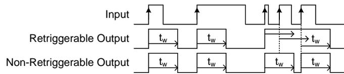
Figure 3. Difference Between Retriggerable and Non-Retriggerable Monostable Multivibrators
