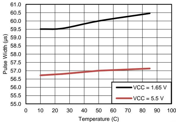
Figure 7. Pulse Width Over Temperature and Supply Voltage Range With C<sub>ext</sub> = 100 pF and R<sub>ext</sub> = 100.7 kΩ
