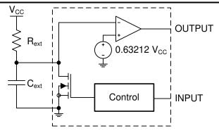
Figure 3-1. Functional Diagram of a Monostable Multivibrator
