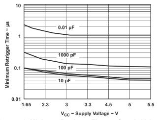
Figure 4-3. Minimum Retrigger Time vs Supply Voltage
