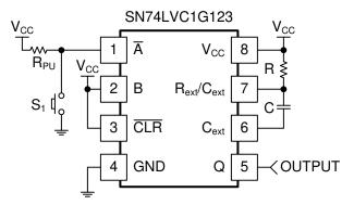
Figure 4-7. Debounce Application Schematic
