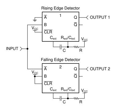
Figure 4-8. Rising and Falling Edge Detector Application Schematic
