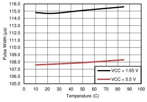
Figure 4-6. Pulse Width Over Temperature and Supply Voltage Range With C<sub>ext</sub> = 1 nF and R<sub>ext</sub> = 100.7 k $\Omega$
