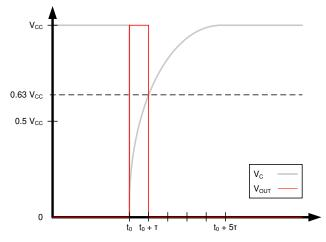
Figure 3-2. Capacitor Voltage With Aligned Output Pulse (Ideal)
