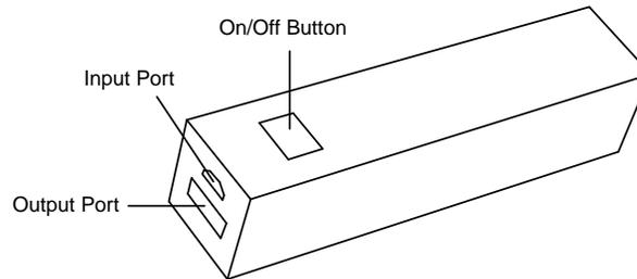
**Figure 1. Typical Power Bank Structure**
