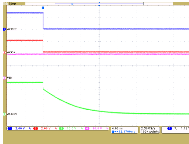
Figure 3. bq24770 Circuit Using EC GPIO1 to Control ACDET, ACDET is Short to GND and ACOK Falls
