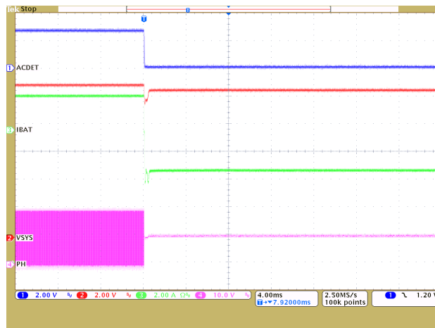
Figure 4. bq24770 Circuit Using EC GPIO1 to Control ACDET, ACDET is Short to GND and Charger Stops Switching
