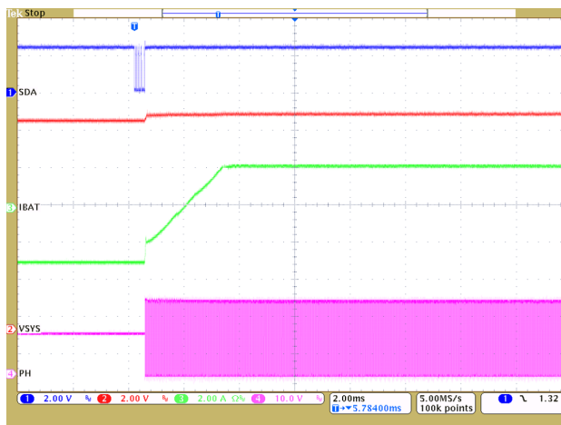
Figure 14. bq24770 Circuit Using LEARN Command, When LEARN is Disabled and Battery Starts Charging
