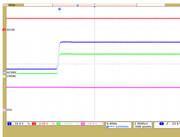
Figure 9. bq24770 Circuit Implementing PPS With ACDRV Control, ACDRV is Released and ACOK Remains High
