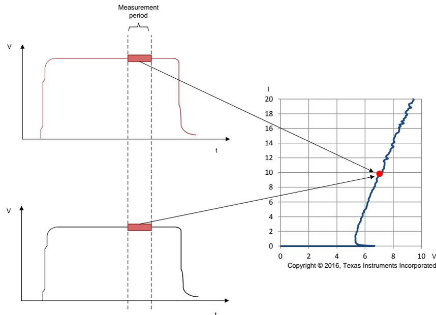
Figure 3. Example IC TLP Results with TPD1E04U04 Superimposed
