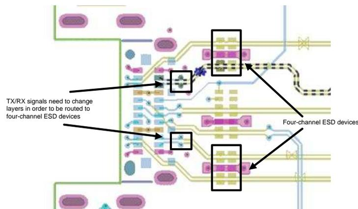
**Figure 6. Example Layout with 4-Channel Routing Inefficiencies**
