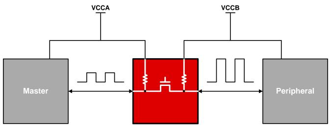
Figure 11. Operation of an I<sup>2</sup>C Voltage Translator/Level Shifter
