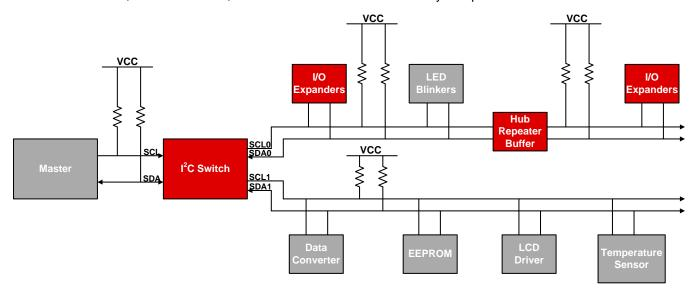
Figure 1. I<sup>2</sup>C Bus With Peripheral Devices Attached Example
