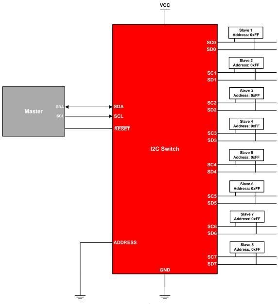
Figure 5. Eight-Channel I<sup>2</sup>C Switch Example
