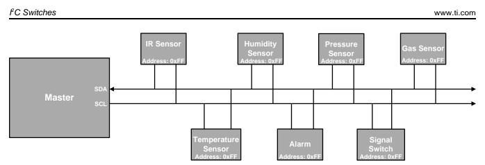
Figure 4. I<sup>2</sup>C bus with multiple slave devices with the same address
