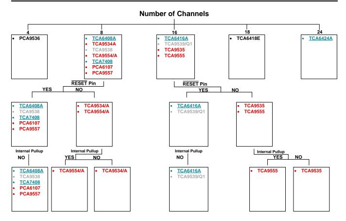
Note: Underlined devices indicate level-shifting ability.
