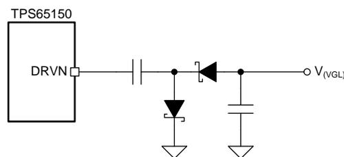
**Figure 1. One-Stage Negative Charge-Pump Circuit**
