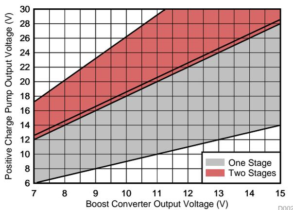
Figure 5. Positive Charge Pump Output Voltage Ranges
