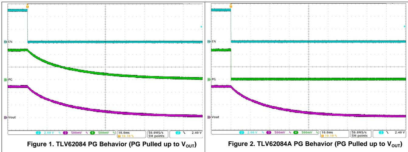
Figure 1. TLV62084 PG Behavior (PG Pulled up to  $V_{OUT}$ )
