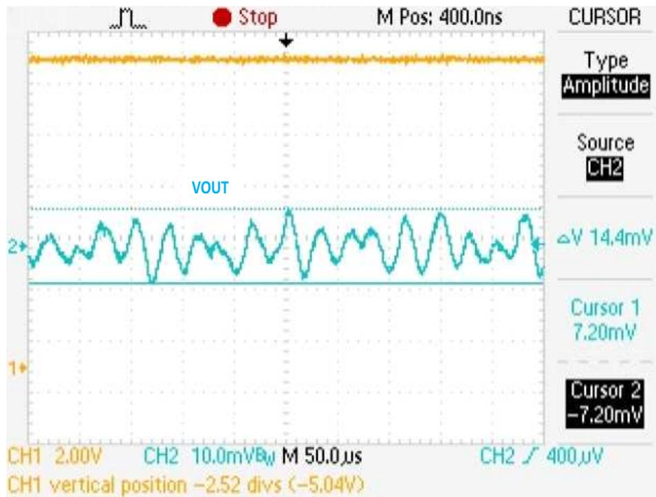
**Figure 14. Effect of Output Capacitance Under a Light Load Condition,**
