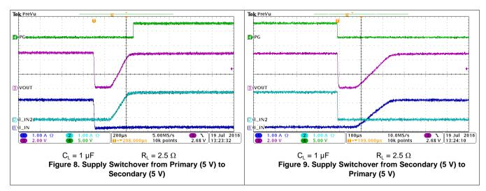
For a break-before-make configuration, taken from Figure 8, a 2-A load will not cause reverse current when transitioning to the secondary power supply as the TPS22953 completely turns off before the secondary load switch fully enables. This can be seen on the output voltage as it drops completely and then it is restored in about 400  $\mu$ s.
