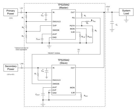
Figure 12. Priority MUXing Circuit with Two TPS25942s
