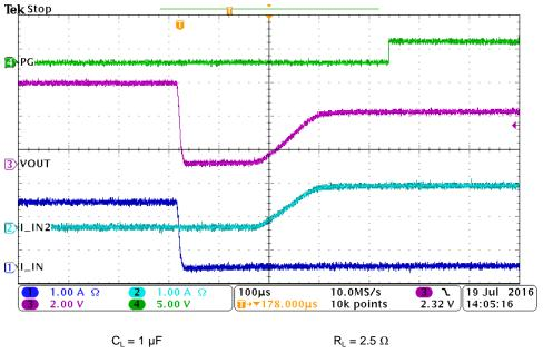
Figure 11. Supply Switchover from Primary (5 V) to Secondary (3.3 V)
