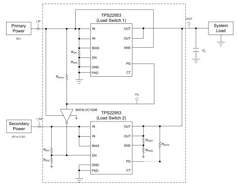
Figure 7. Break-Before-Make Power MUXing Circuit Using Two TPS22953s
