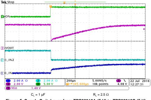
Figure 5. Supply Switchover from TPS22910A (5 V) to TPS22912C (5 V)
