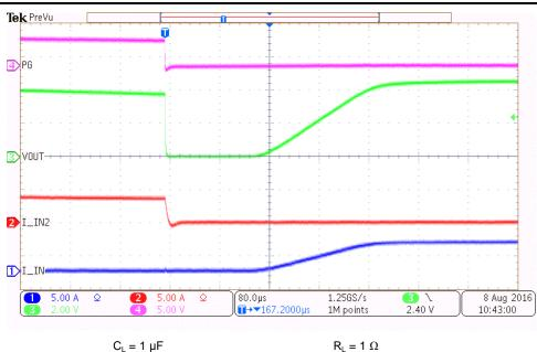
Figure 10. Supply Switchover from Primary (5 V) to Secondary (5 V) with 5 A
