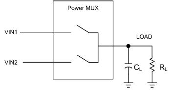
Figure 1. Power MUXing Block Diagram
