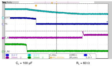
Figure 15. Supply Switchover from Primary (12 V) to Secondary (5 V)
