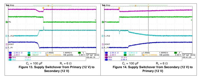
For the 12-V rails in Table 5, the voltage drops for each case can be compared to one of a diode as the "diode mode" of the TPS25942 is utilized. In some configurations, the input current does not reflect a large inrush current as a result of the lower capacitive loads.
