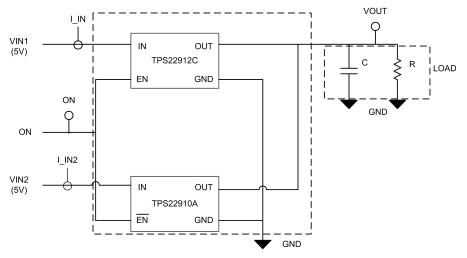
Figure 4. Power MUXing With the TPS22910A and TPS22912C
