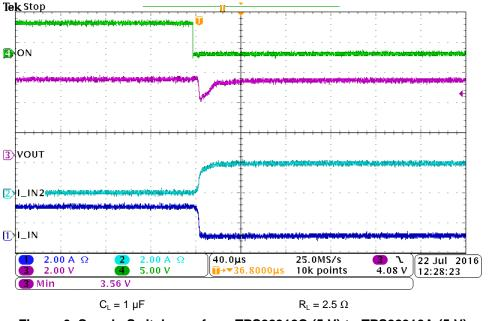
Figure 6. Supply Switchover from TPS22912C (5 V) to TPS22910A (5 V)
