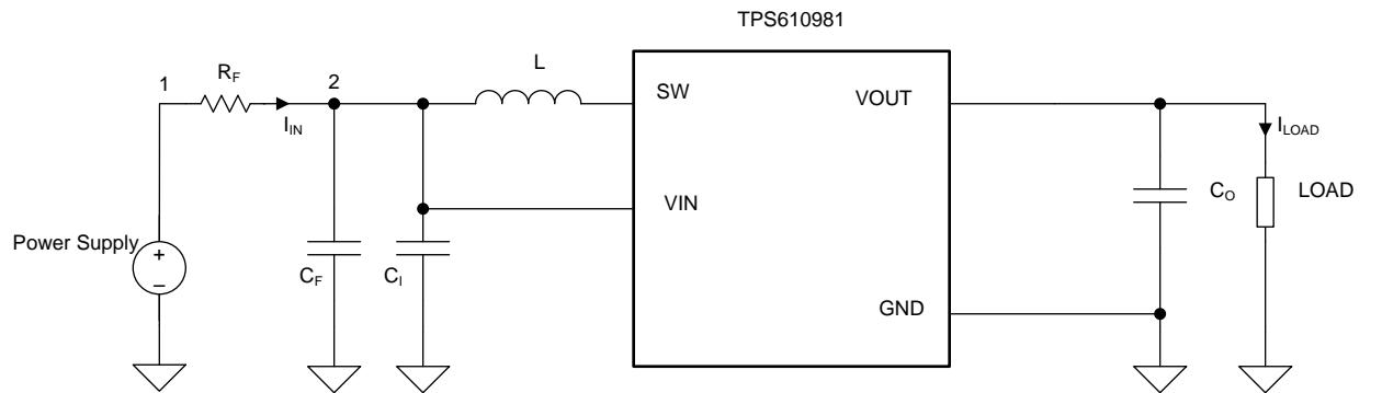
**Figure 5. Method to Measure the No Load Input Current**
