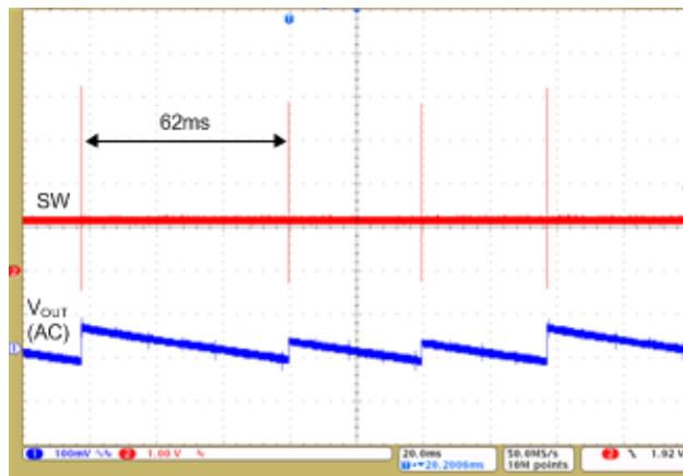
**Figure 4. Switching Frequency at No Load Condition**
