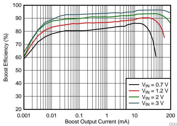
**Figure 3. Efficiency of TPS610981 at Low Power Mode**
