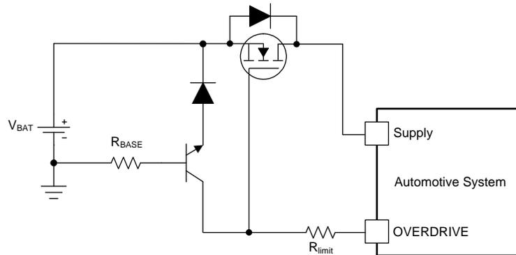
Figure 5. Reverse Battery Protection With BJT and NMOS
