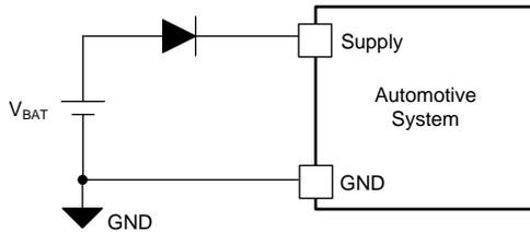
Figure 1. Reverse Battery Protection With Diode at Supply Terminal
