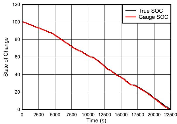
**Figure 3. Reported SOC vs. True SOC Under Highly Dynamic Battery Voltage and Current**
