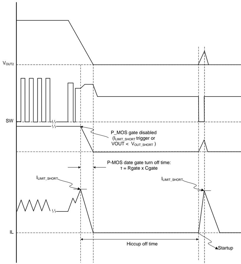
**Figure 2. TPS61178x Hiccup Mode Protection Timing Diagram**
