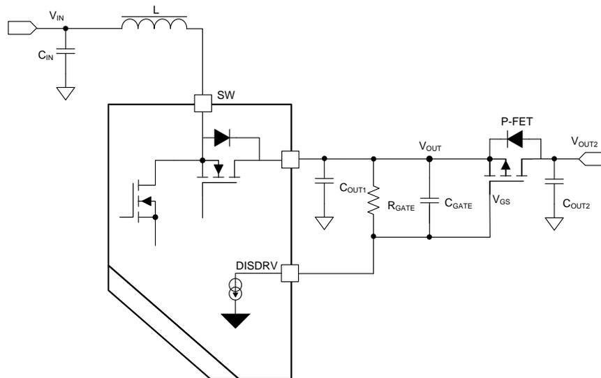
**Figure 1. TPS61178x Application Circuit with External P-FET**
