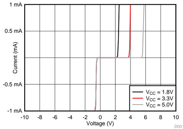
Figure 2. BAV99 I-V Curve (Multiple  $V_{CC}$ s)
