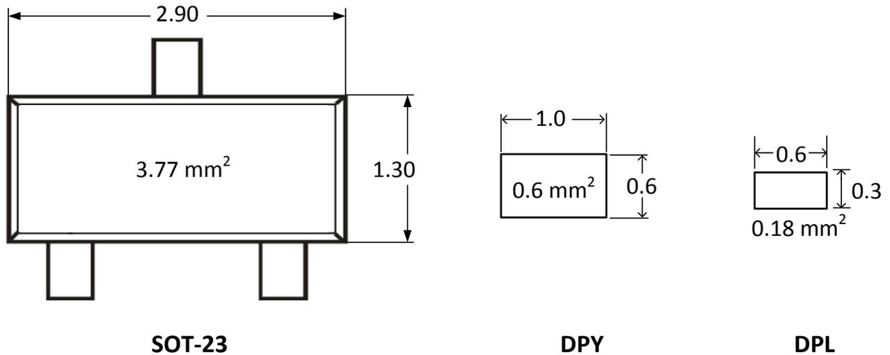
Figure 8. SOT23 Package vs DPY and DPL Package
