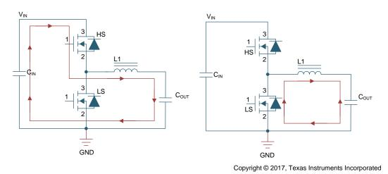
Figure 2. AC Current Flow
