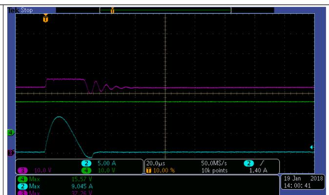
Figure 11. TVS3300 From TI Protection at 9 A at 85°C
