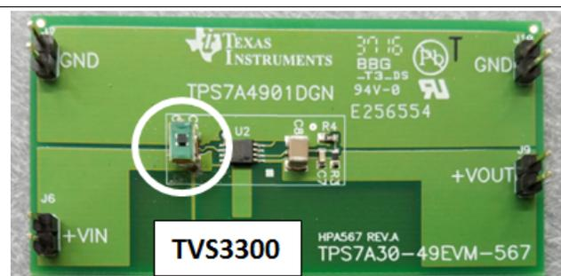
Figure 8. TPS7A4901DGN with TVS3300 on the Input Voltage Line
