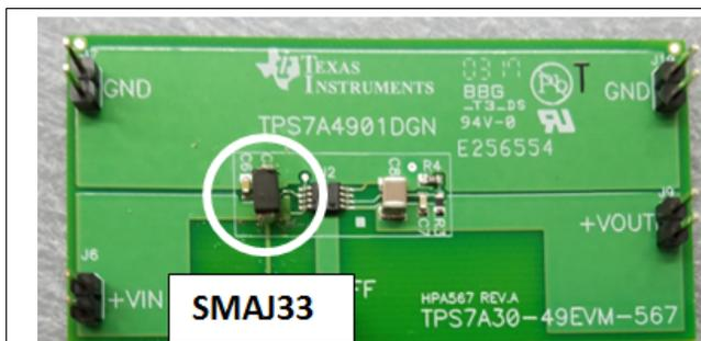
Figure 7. TPS7A4901DGN with SMAJ33A on the Input Voltage Line
