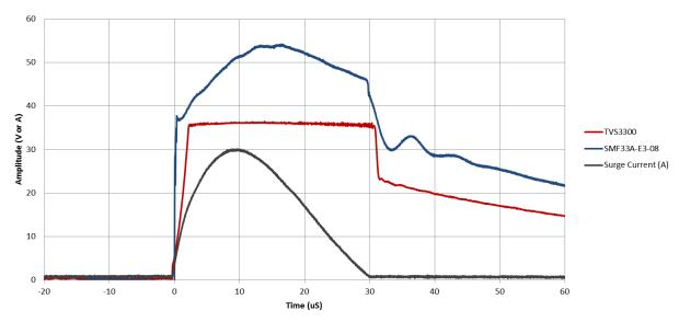
Figure 5. 8/20 µs Surge Clamping Waveform of Flat-Clamp Diode vs. Conventional TVS Diode
