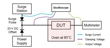
Figure 9. Test Setup Block Diagram
