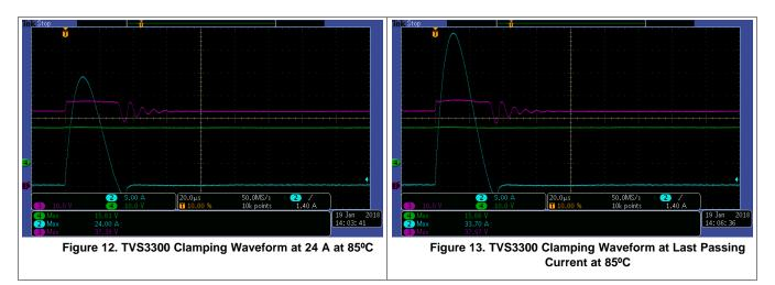
It is clear that the Flat-Clamp TVS3300 provides more robust protection for the input to this piece of equipment than conventional TVS diodes. The very low  $R_{\text{DYN}}$  of the TVS3300 enables using the 36-V absolute maximum LDO. If a traditional TVS diode is used, the selected TPS7A49 device must be swapped with a device that is rated for 60 V or higher input tolerance, increasing cost and complexity of the design.
