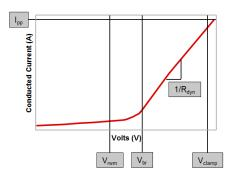
Figure 1. Stand-off, Break Down and Clamp Voltage
