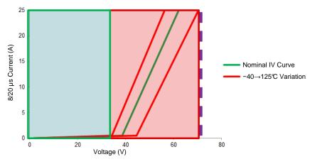
Figure 2. Process and Temperature Variation on SMAJ33A
