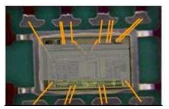
Figure 1. Bonding Wire Package Top View
