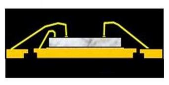
Figure 2. Bonding Wire Package Cross-Sectional View
