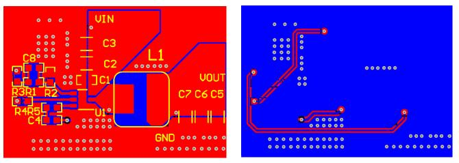
Figure 6. Top PCB Layout
