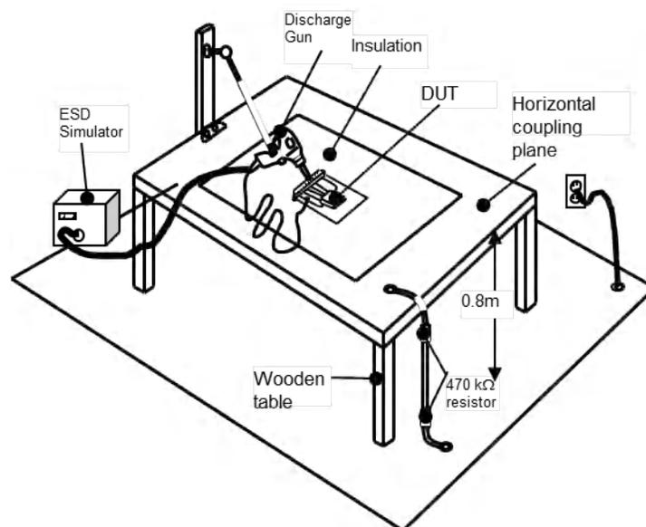
**Figure 3-1. ISO 10605 Basic Table Setup**
