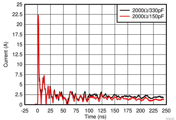
**Figure 2-3. 2000-Ω, 5-kV Contact Discharge**
