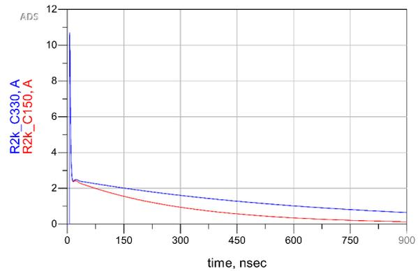
**Figure 2-5. 2000-Ω, 5-kV Contact Discharge Ideal Current Waveform**
