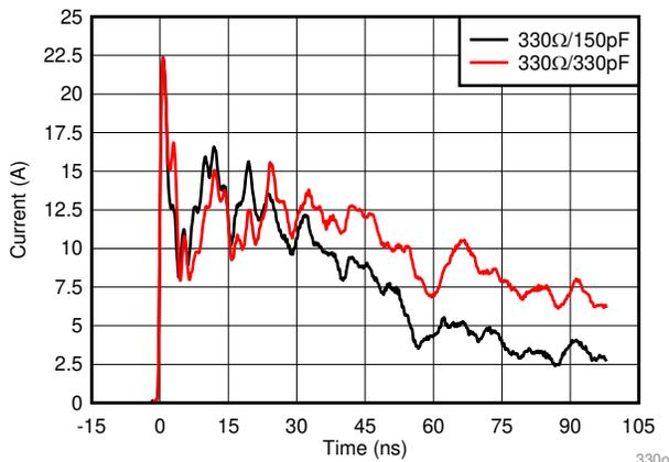
**Figure 2-2. 330-Ω, 5-kV Contact Discharge**
