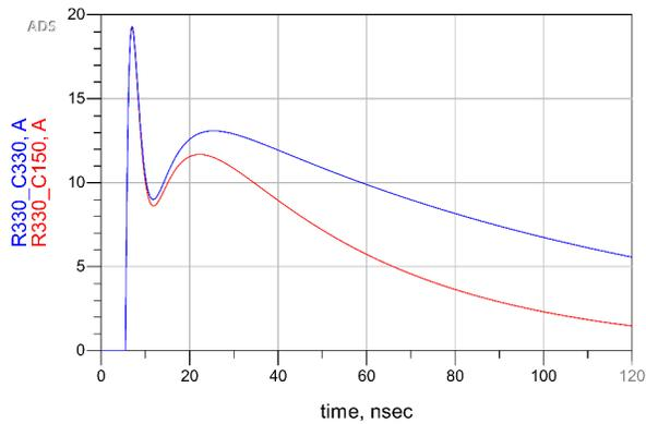
**Figure 2-4. 330-Ω, 5-kV Contact Discharge Ideal Current Waveform**
