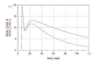
Figure 2-4. 330-Ω, 5-kV Contact Discharge Ideal Current Waveform
