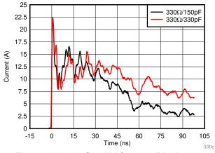
Figure 2-2. 330-Ω, 5-kV Contact Discharge
