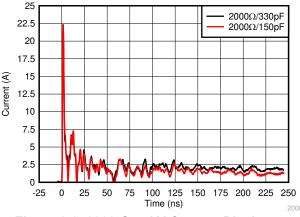
Figure 2-3. 2000-Ω, 5-kV Contact Discharge
