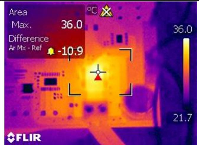
Figure 16. Multi-Chip Module Internal-FET Topology With Steady-State 3-A Load
