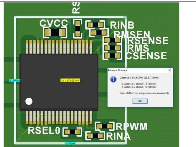
Figure 9. High Current Multi-Chip Module Internal-FET Example
