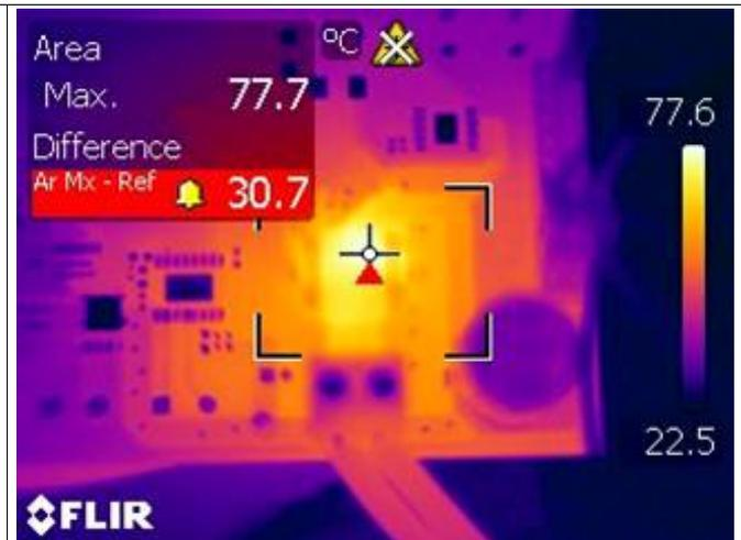
Figure 18. Multi-Chip Module Internal-FET Topology With Steady-State 6-A Load
