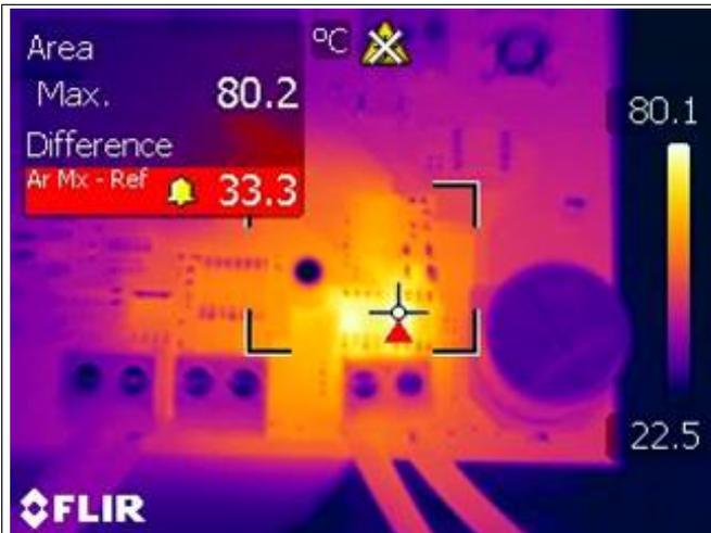
Figure 17. Gate Driver External-FET Topology With Steady-State 6-A Load
