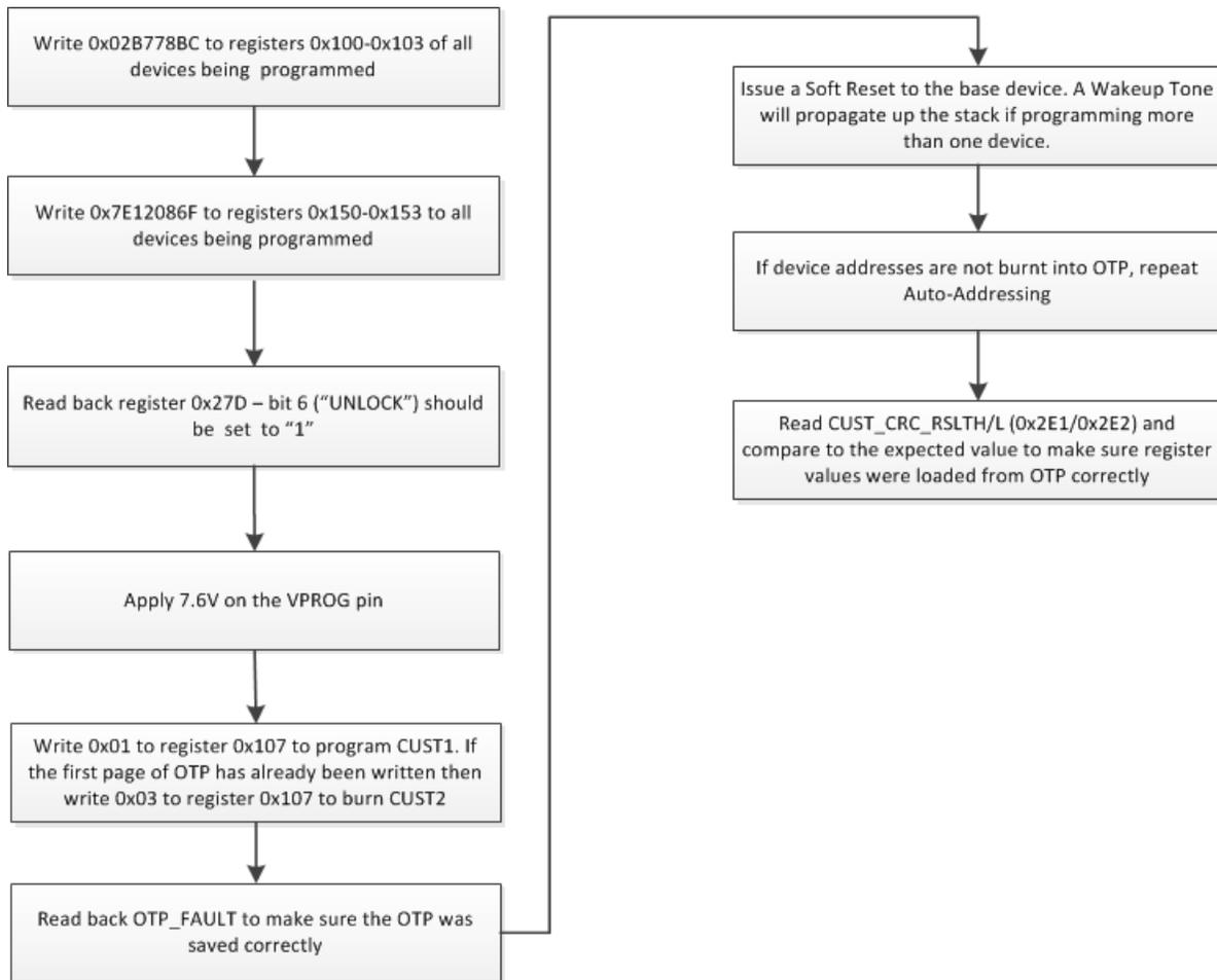
**Figure 5. OTP Programming Flowchart**
