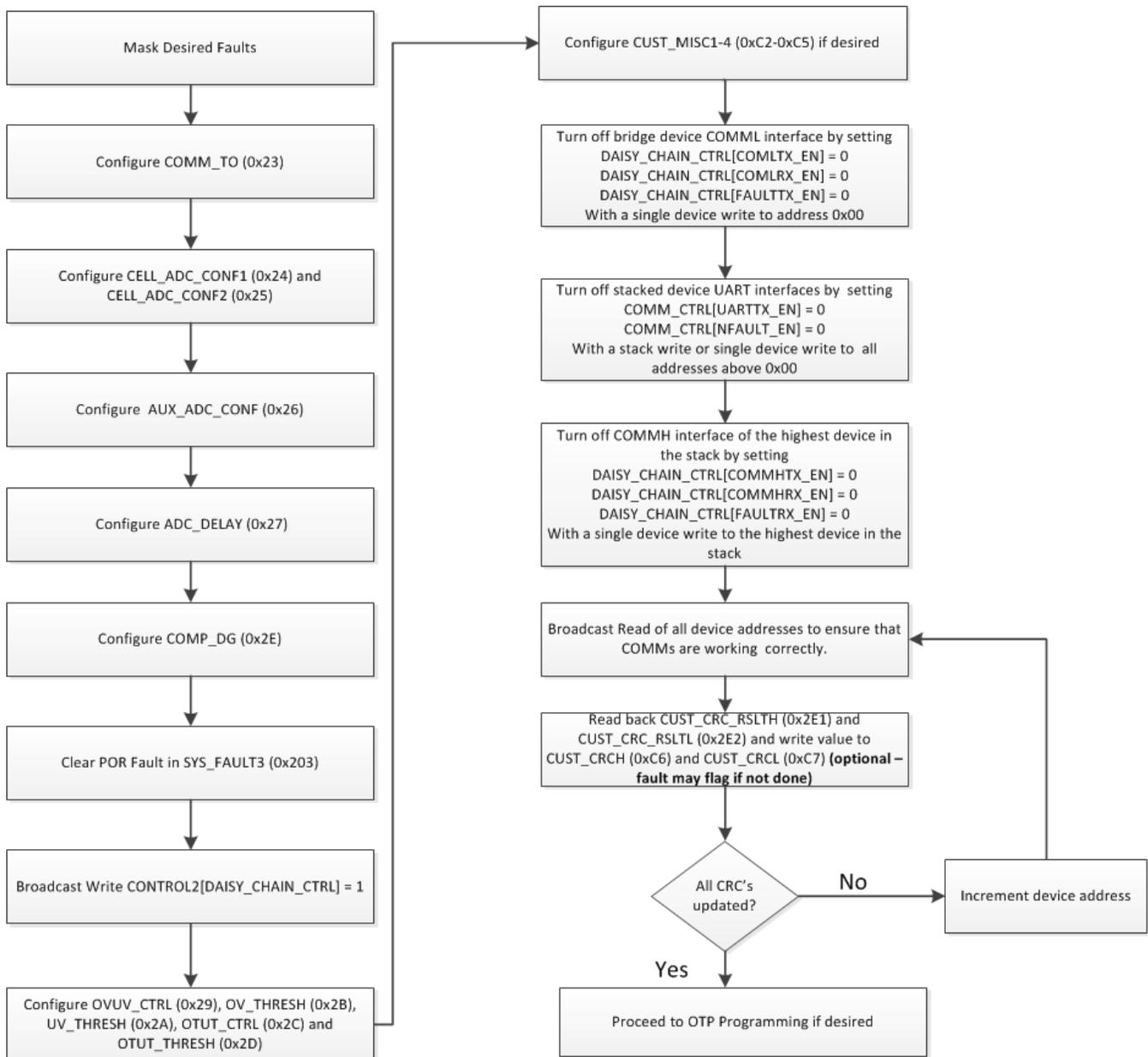
Figure 4. Generic Register Initialization Procedure
