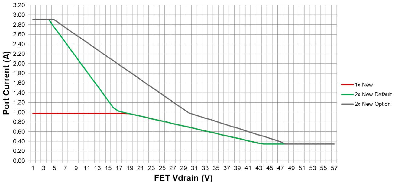
Figure 3. New ILIM Protection Curve of the TPS23880
