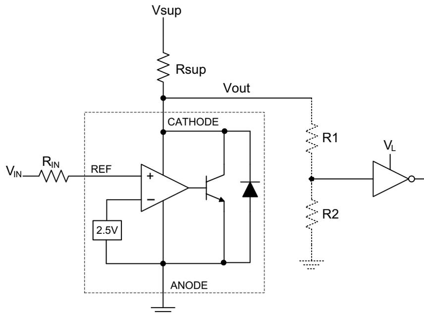
Figure 1. Voltage Comparator Application Functional Block Diagram
