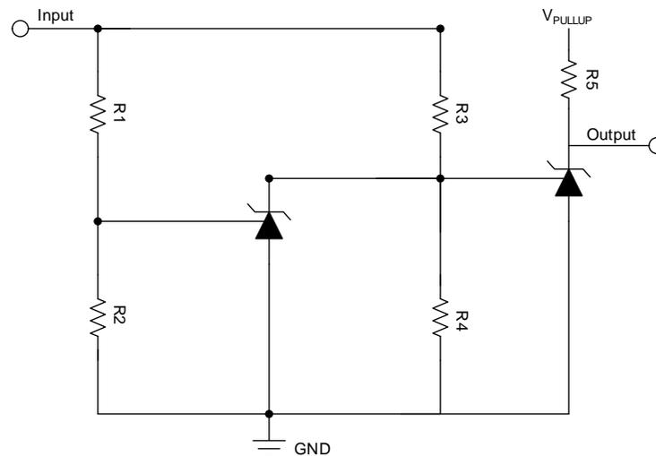
Figure 3. Window Comparator Application Schematic
