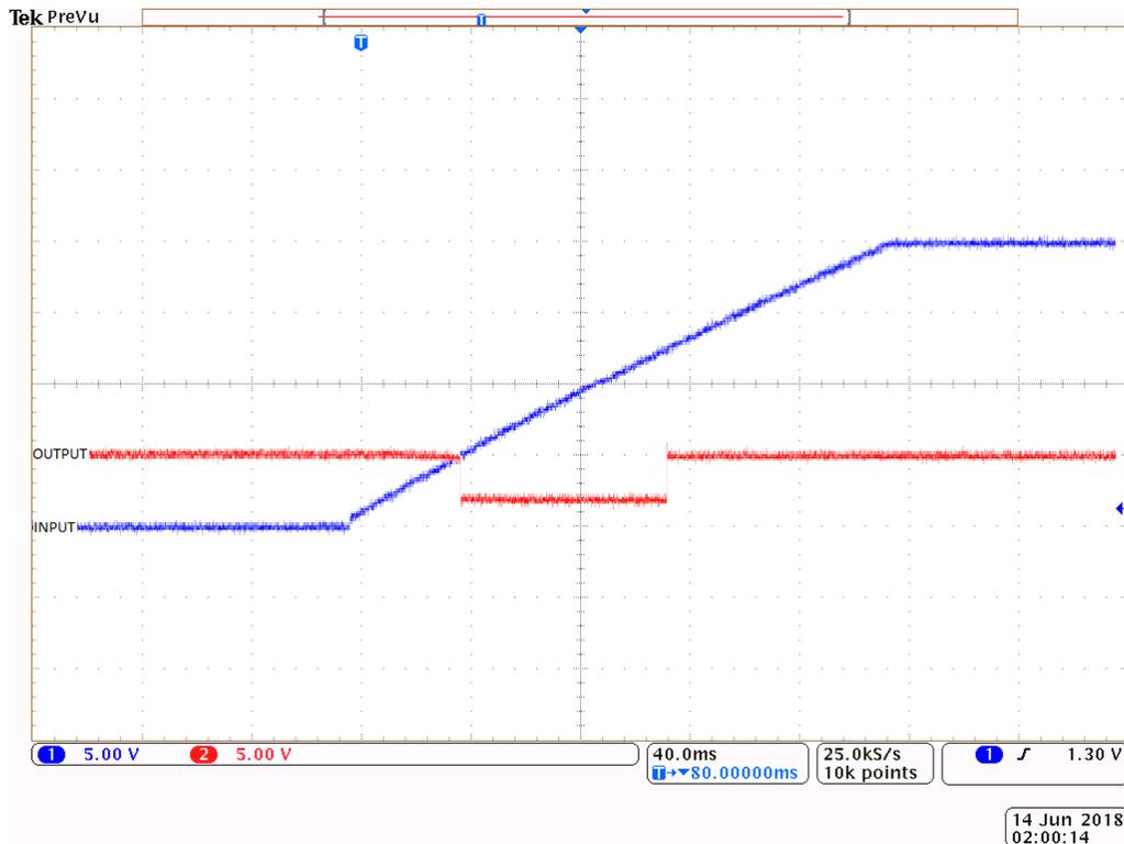
Figure 4. Window Comparator Output
