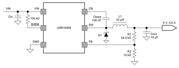
Figure 6. Application Circuit with 5-V Output DC/DC the LMR16006
