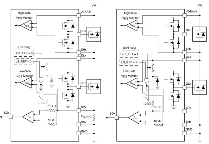
Figure 4. Resistor Sense Configuration
