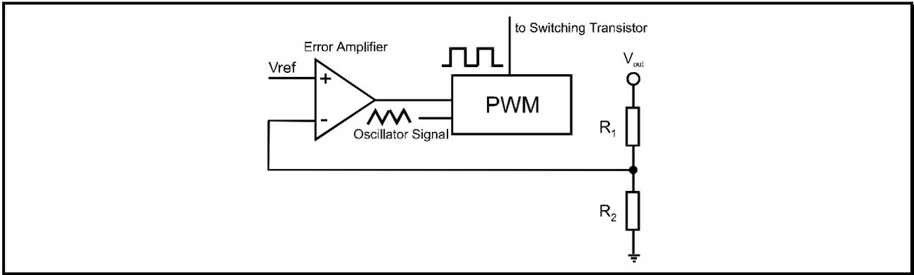
**Figure 5.1:** Schematic diagram of a pulse width modulator
