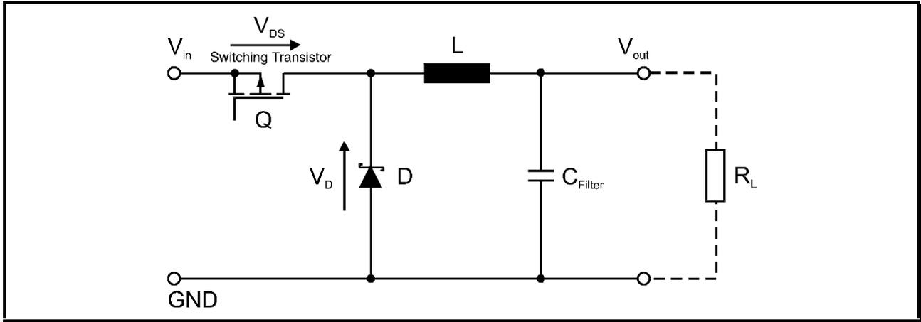
**Figure 2.1:** Schematic diagram of a Step-Down Converter
