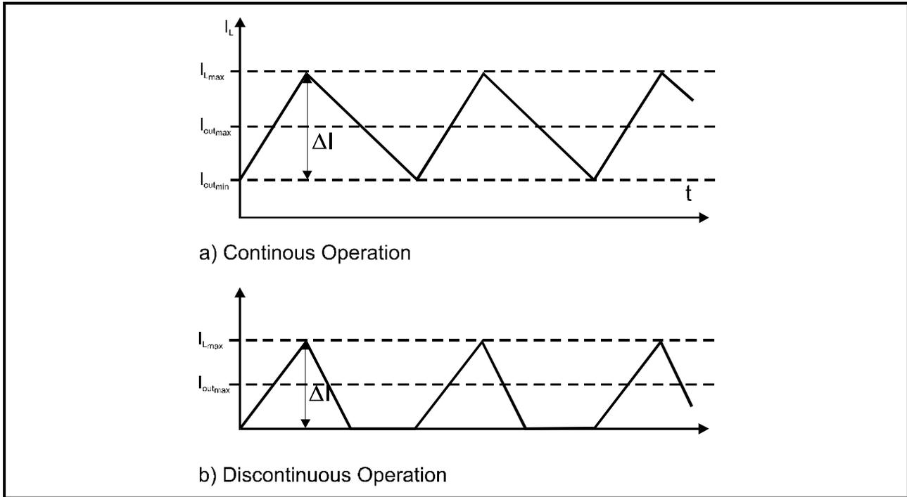
**Figure 2.2: Inductor current, with continuous and discontinuous operation**
