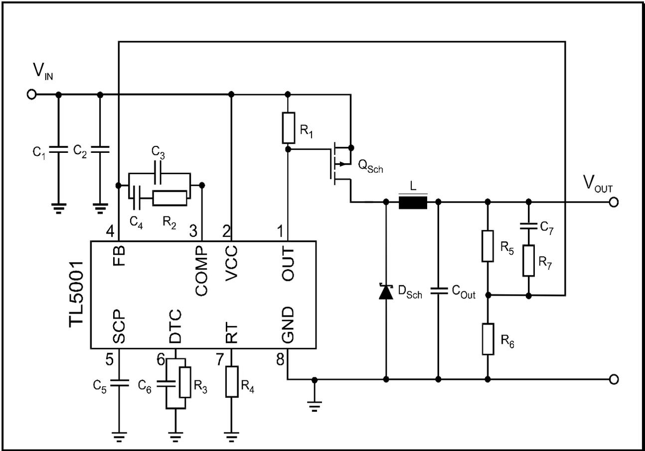
**Figure 10.2:** Step-Down Converter for low output currents
