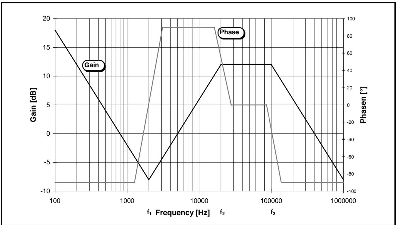
**Figure 7.5: Bode diagram of the compensating network**
