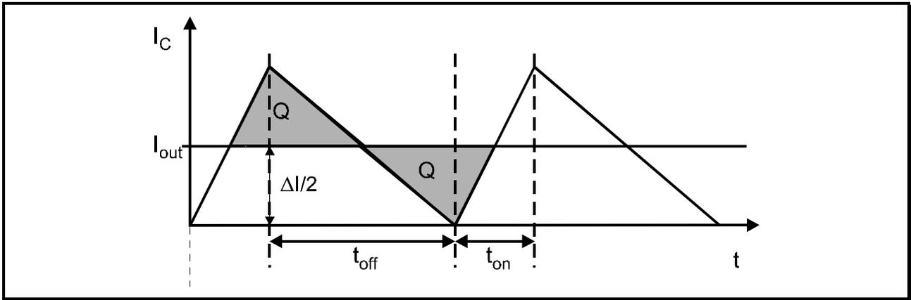
**Figure 2.4:** Curve of current in the capacitor
