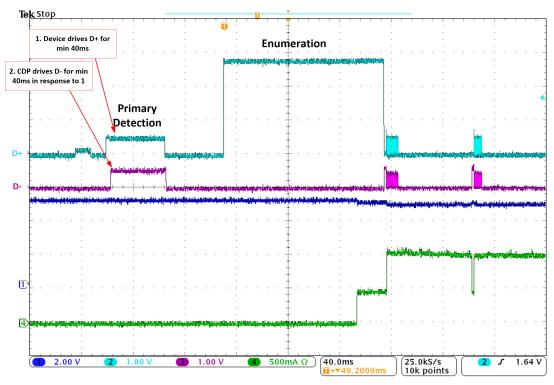
Figure 1. BC1.2 CDP Process Example
