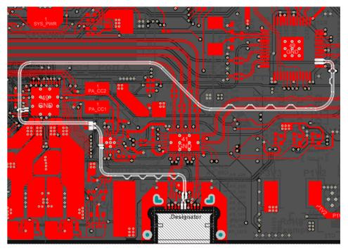
Figure 7. TPS65987D/88 D+/D- Routing Example with BC1.2 Support
