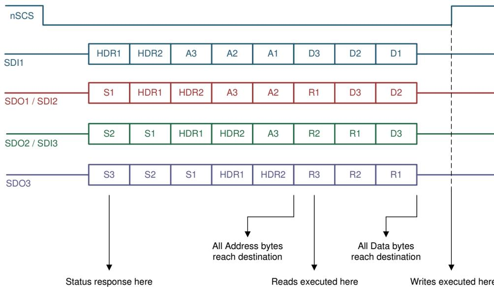
Figure 3-1. SPI Frame With Three Motor Driver (Peripheral) Devices
