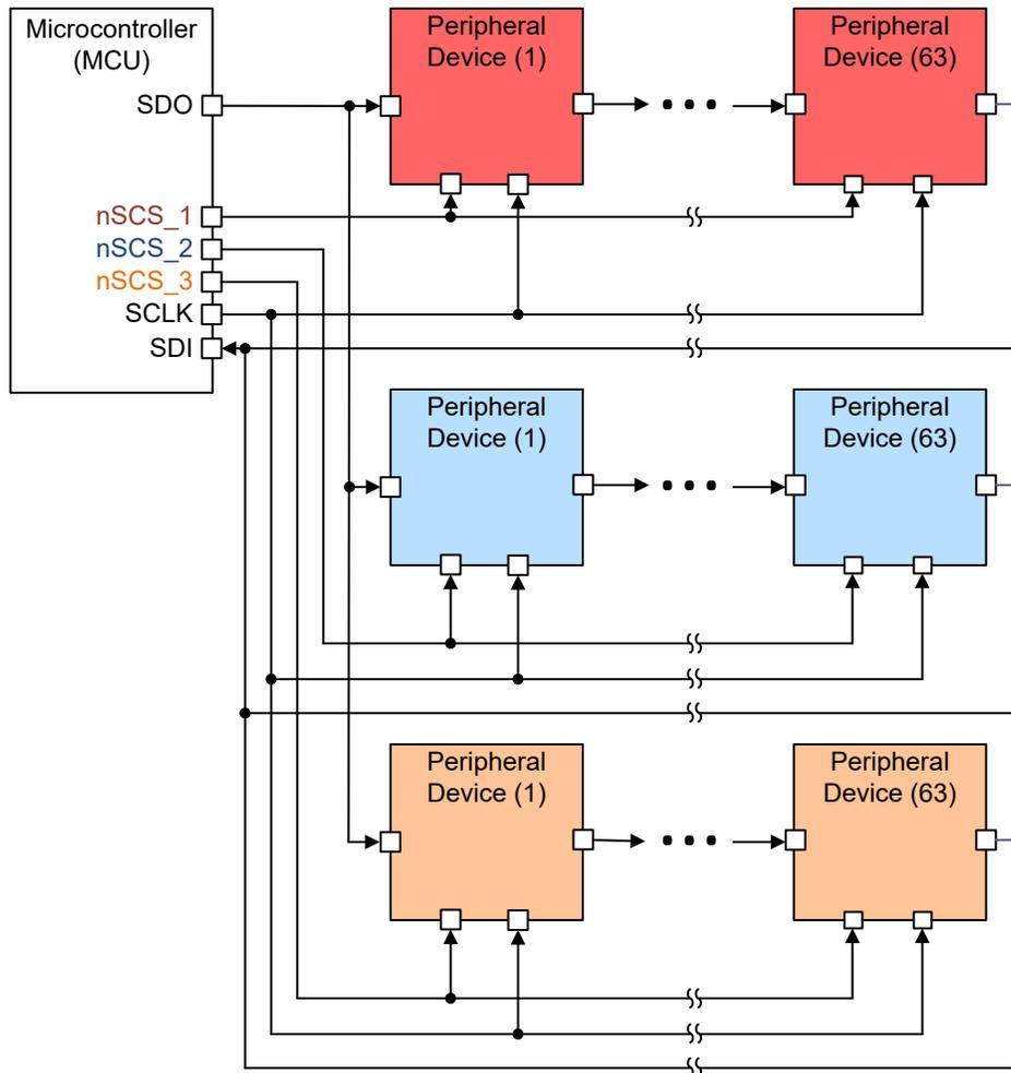
Figure 4-6. SPI Block Diagram for Controlling More Than 63 Devices
