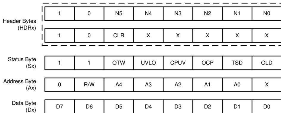
**Figure 3-3. Contents of Header, Status, Address, and Data Bytes**
