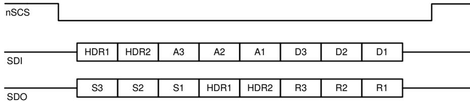
**Figure 3-4. SPI Data Sequence between MCU and Three Motor Driver Devices**
