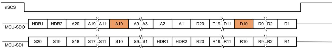
**Figure 4-2. SPI Daisy Chain Data Frame for 20 Devices**
