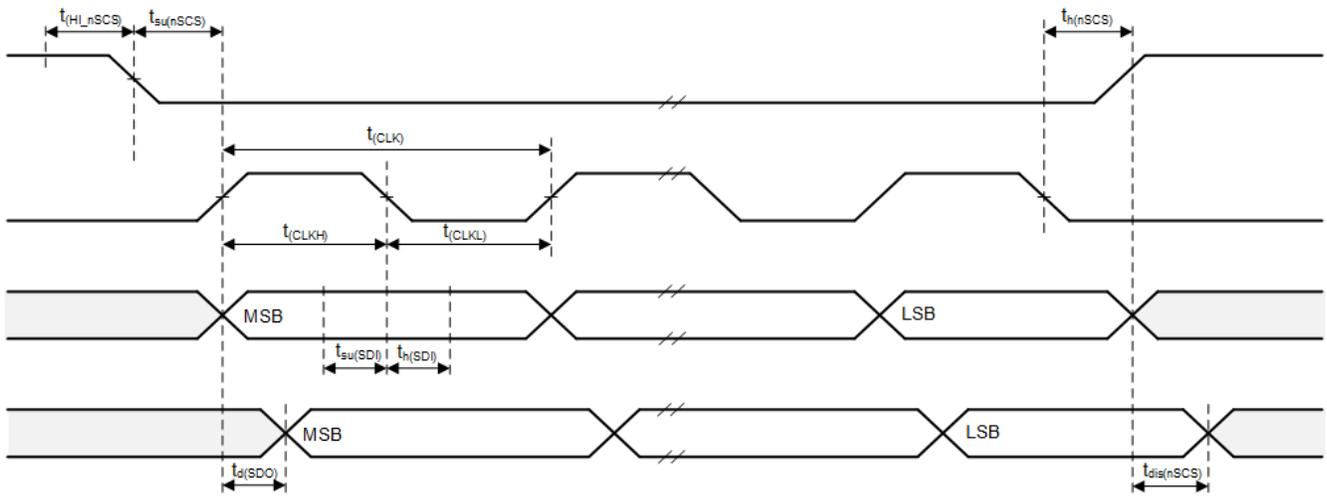
Figure 4-5. SPI Frame Timing Diagram from DRV8889-Q1 Datasheet
