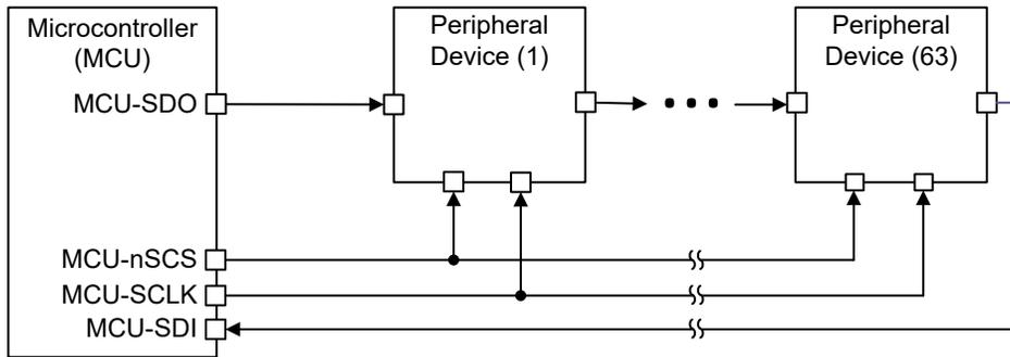
Figure 4-3. SPI Daisy Chain Block Diagram for 63 Devices
