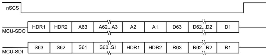
Figure 4-4. SPI Daisy Chain Data Frame for 63 Devices
