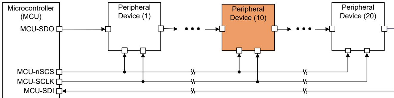
**Figure 4-1. SPI Daisy Chain Implementation Example for 20 Devices**
