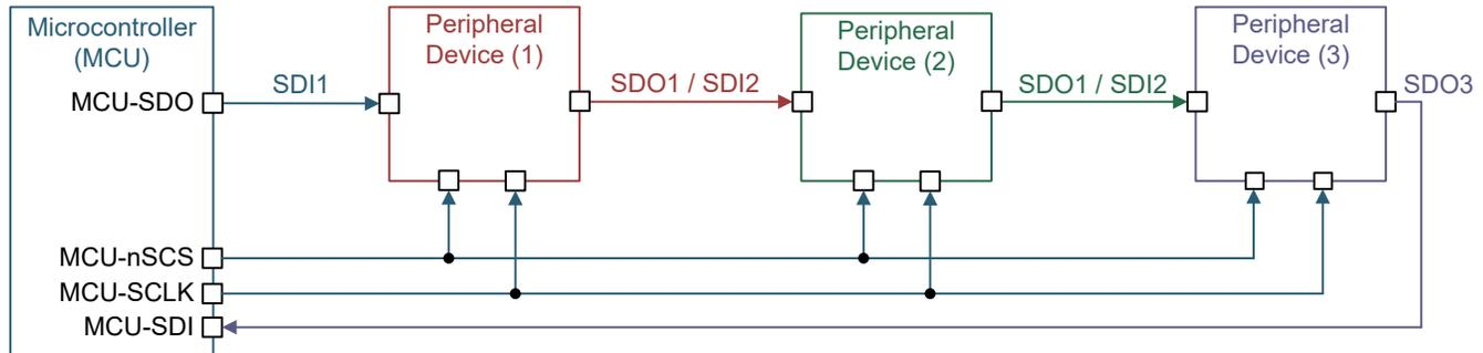
**Figure 2-1. Three Motor Driver Devices Connected in Daisy Chain**
