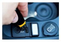
Media interface refers to the system that connects external or internal media (from a cellphone, media player, and so forth) to the vehicles infotainment system, while head unit refers to the hardware interface of an automotive infotainment system.
