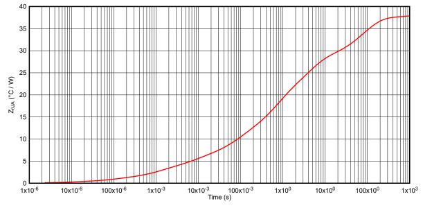
Figure 6-8. TPS1HB50-Q1 Transient Thermal Impedance  $Z_{\Theta JA}$
