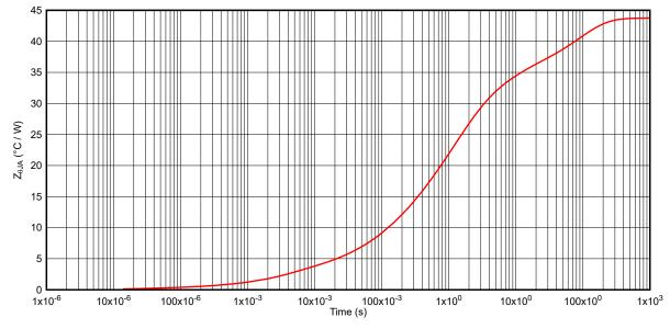
Figure 6-4. TPS1H100-Q1 Transient Thermal Impedance  $Z_{\Theta JA}$
