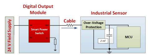
Figure 3-2. Industrial Capacitive Load Driving Example
