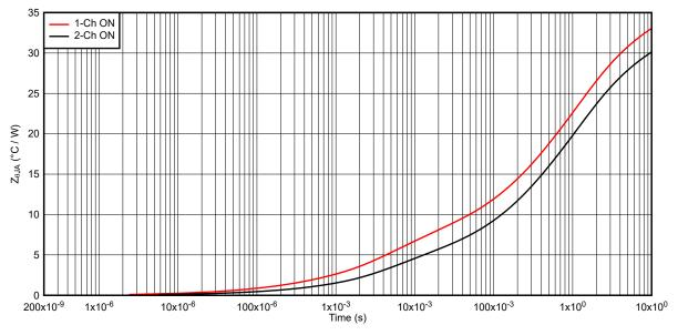
Figure 6-6. TPS2H160-Q1 Transient Thermal Impedance  $Z_{\mbox{\scriptsize OJA}}$
