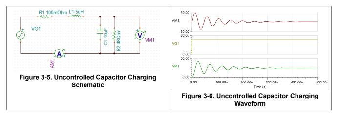
Figure 3-6 shows that an uncontrolled dV/dT leads to an inrush current that reaches nearly 30A with severe ringing. Without current limiting this is the quickest way to charge the capacitor, however for many systems this sort of inrush current is not acceptable and cannot be supported by the input power rail.
