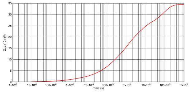
Figure 6-12. TPS1HB16-Q1 Transient Thermal Impedance  $Z_{\Theta JA}$
