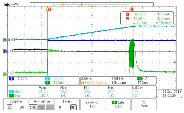
Figure 3-9. TPS2H160-Q1 Current Limiting at 1A
