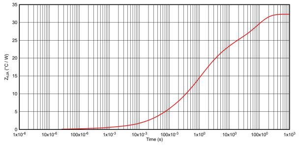
Figure 6-14. TPS1HA08-Q1 Transient Thermal Impedance  $Z_{\Theta JA}$
