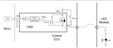
Figure 5-3. Open Load Detection Schematic
