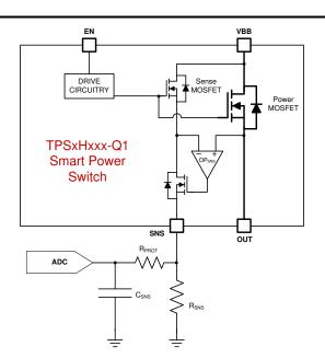
Figure 2-3. TPSxHxxx Current Sense Circuit
