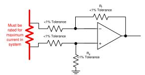
Figure 2-2. Discrete Current Measurement Implementation
