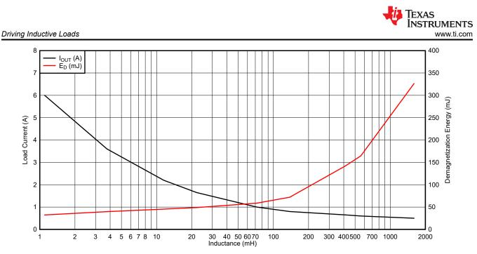
Figure 4-5. TPS4H160-Q1 Demagnetization Capability
