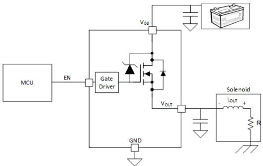
Figure 4-1. Solenoid Application Example
