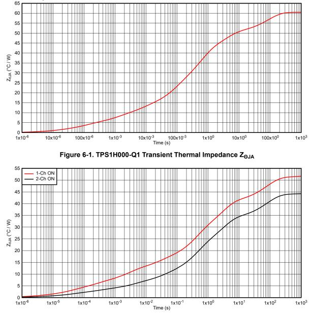
Figure 6-2. TPS2H000-Q1 Transient Thermal Impedance  $Z_{\Theta JA}$
