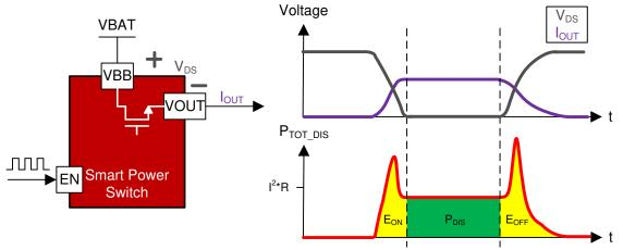
Figure 2-5. Switching Energy Losses during PWM
