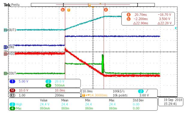
Figure 3-11. V<sub>DS</sub> While Charging Capacitance
