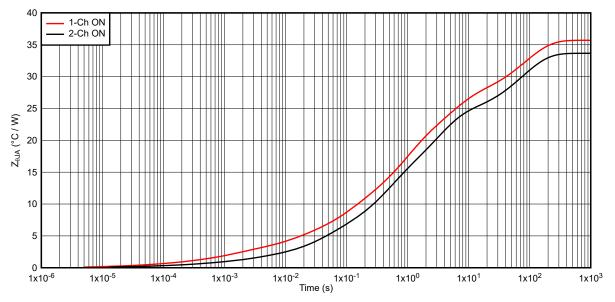
Figure 6-11. TPS2HB35-Q1 Transient Thermal Impedance  $Z_{\Theta JA}$
