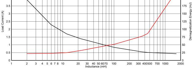
Figure 6-18. TPS2HB50-Q1 Demagnetization Energy Capability
