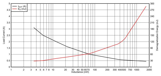
Figure 6-16. TPS1H200-Q1 Demagnetization Energy Capability
