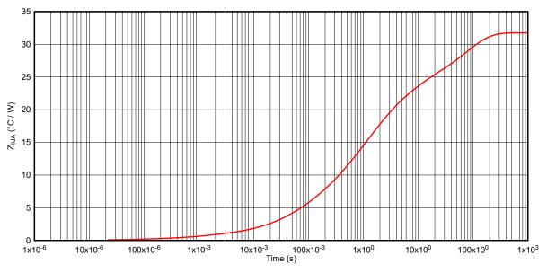
Figure 6-15. TPS1HB08-Q1 Transient Thermal Impedance  $Z_{\Theta JA}$
