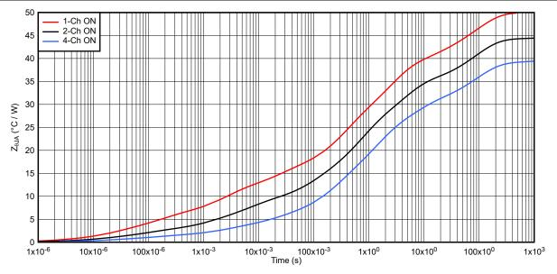
Figure 6-3. TPS4H000-Q1 Transient Thermal Impedance  $Z_{\mbox{\scriptsize OJA}}$
