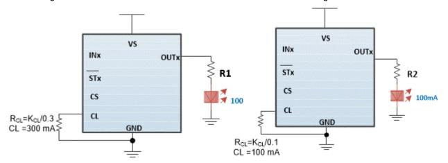
Figure 5-4. Driving LED in Constant Output Voltage and Constant Current Mode
