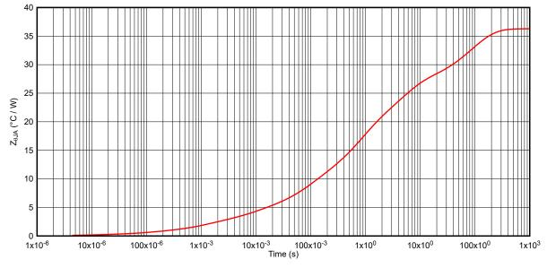
Figure 6-10. TPS1HB35-Q1 Transient Thermal Impedance  $Z_{\Theta JA}$
