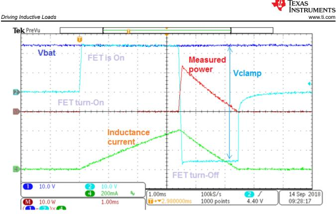
Figure 4-4. Demagnetization Energy During Inductive Turn-Off
