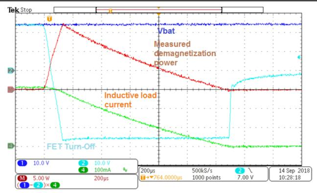
Figure 4-6. Load 1 Measured Demagnetization Energy
