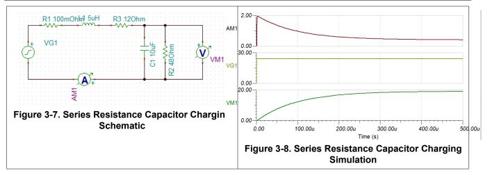
The addition of a  $12\Omega$  current limiting resistor limits the peak current to less than 2A, but is not a viable solution due to the power dissipation and voltage drop over the additional  $12-\Omega$  resistance. With a 500mA DC load this adds 3W of additional power dissipation and a 6V drop over the resistor. This heat dissipation and voltage drop are not acceptable in the majority of applications.
