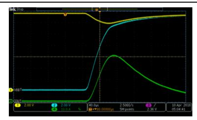
Figure 3-4. Inrush Supply Droop Example
