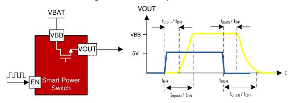
Figure 2-4. Smart High Side Switching Waveform
