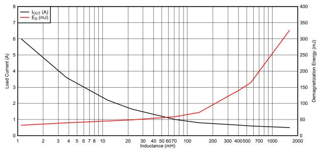
Figure 6-20. TPS4H160-Q1 Demagnetization Energy Capability
