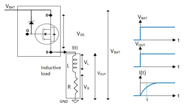
Figure 4-2. Inductive Load Turn-On Phase
