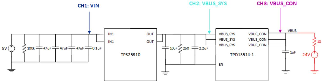
**Figure 2. Test Configuration**
