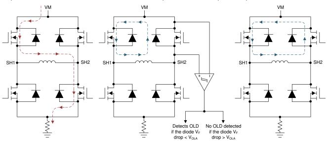
Figure 3-4. Circuit for Active OLD in a DRV8873-Q1 and in a DRV8873 device
