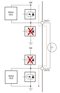
Figure 1-6. Active OLD for Load Connected in H-Bridge Configuration
