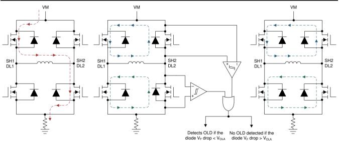
Figure 3-6. Circuit for Active OLD in a BLDC Gate Driver
