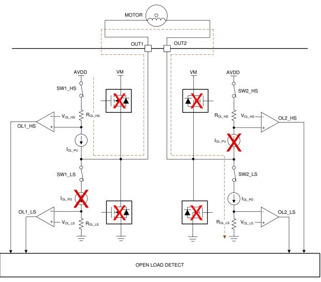
Figure 2-1. Passive OLD Circuit in an Integrated Driver
