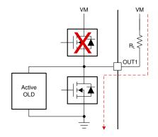
Figure 1-1. Passive OLD for Load Connected to VM
