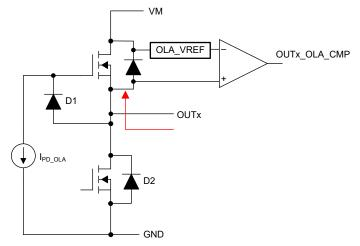
Figure 3-5. Circuit for Active OLD in a DRV824x-Q1 device
