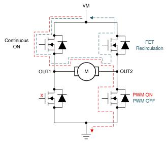
Figure 5-1. Forward Drive and Braking in Synchronous Rectification
