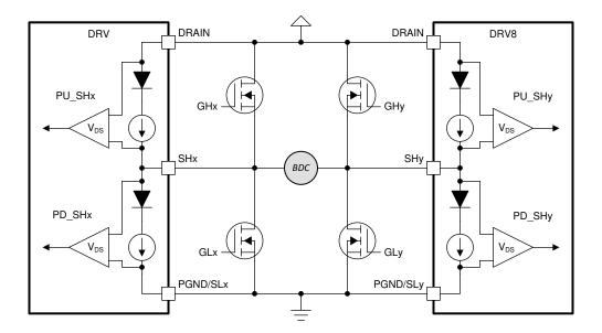
Figure 2-2. Passive OLD Circuit in a Brushed DC Gate Driver
