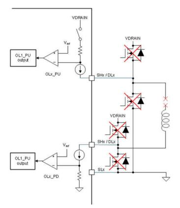
Figure 2-3. Passive OLD Circuit in a Brushless DC Gate Driver
