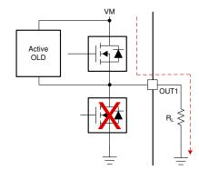
Figure 1-3. Passive OLD for Load Connected to GND
