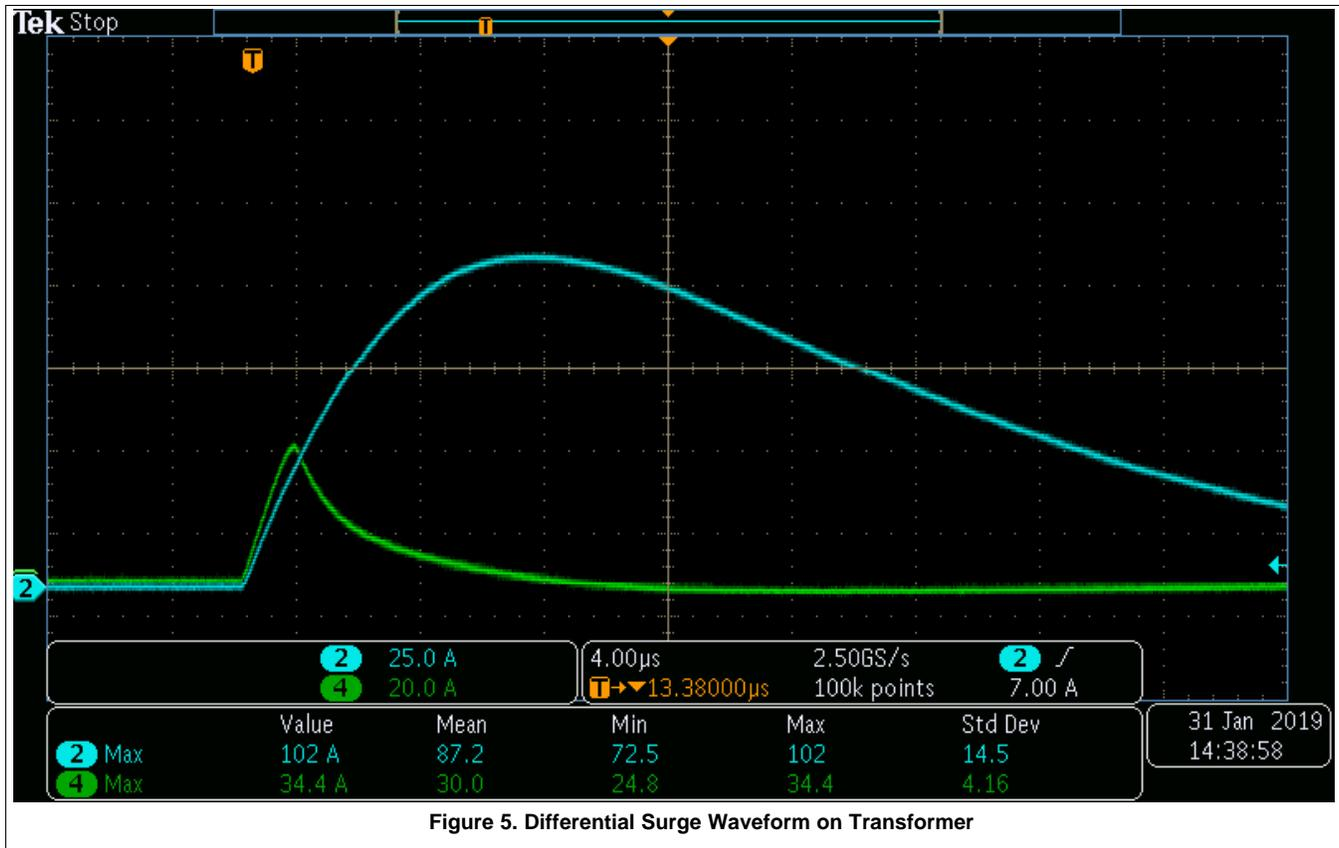
Figure 5. Differential Surge Waveform on Transformer
