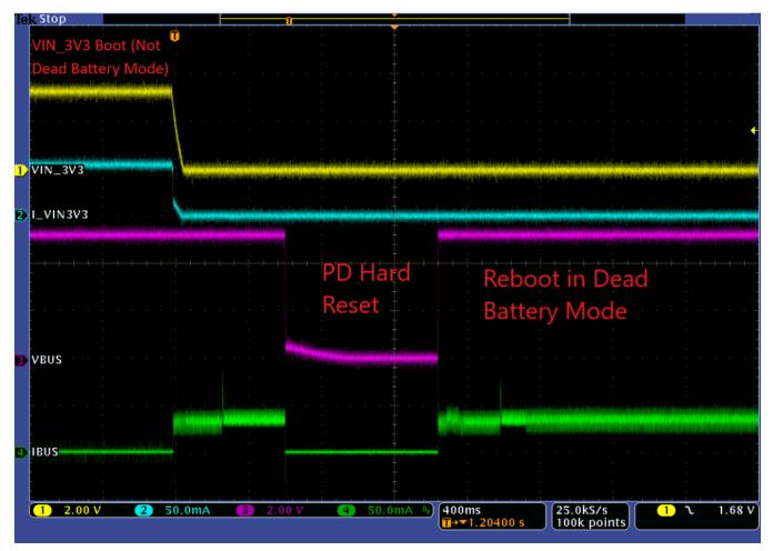
Figure 4. VIN\_3V3 to VBUS LDO Supply Switchover
