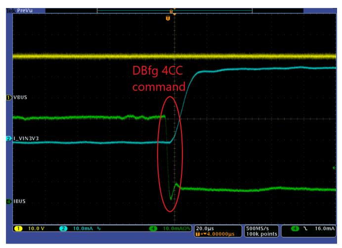
Figure 3. VBUS LDO to VIN\_3V3 Supply Switchover
