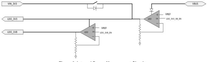
Figure 2. Internal Power Management Circuitry
