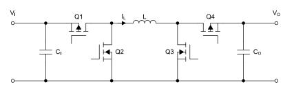
Figure 2. Non-inverting Buck-Boost Converter Schematic
