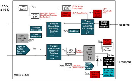
Figure 1. Block Diagram Example of an Optical Module
