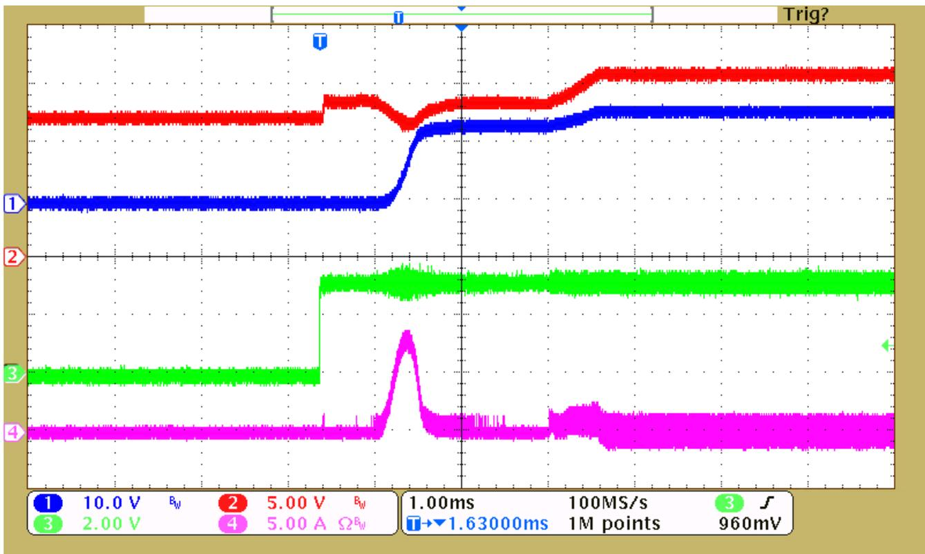
Usually, these loop compensation components are chosen based on the stability in normal operation, but for this device, the components also affect inrush current during start-up. With a lower resistor (from COMP pin to GND), the inrush current of the initial cycles during start-up can be lowered.
