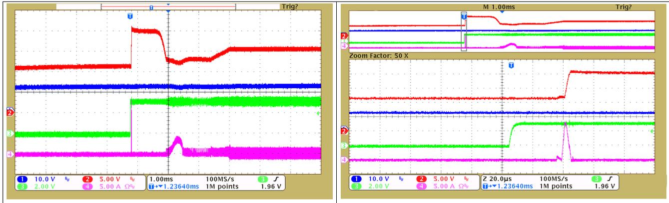
Test condition:  $C_{out}$  before ISO FET is  $4 \times 22\ \mu\text{F}$  (two in parallel and two in series),  $R_c = 39.2\ \text{k}$ ,  $C_c = 1.5\ \text{nF}$ ,  $R_g = 39.2\ \text{k}$ ,  $C_g = 10\ \text{nF}$
