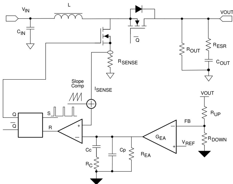
Figure 2. TPS61178x Control Loop of Normal Operation
