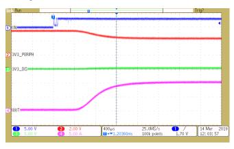
Figure 5. Discrete FET: Power into Short (Damages Discrete FET)
