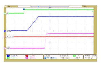
Figure 6. TPS22919: Power into Short (Limits to 500 mA)
