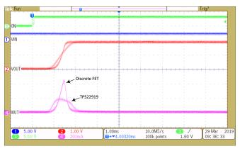
Figure 2. TPS22919 vs Discrete FET Inrush Current Control
