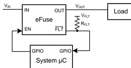
Figure 9. Using a System Microcontroller to Control Fault Response of the eFuse
