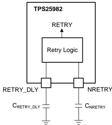
Figure 11. User Adjustable Auto-Retry Scheme Using Two Capacitors
