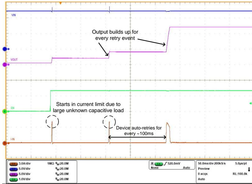
$R_{ILIM} = 332 \Omega$        $C_{OUT} = 2.2 \text{ mF}$        $C_{RETRY\_DLY} = 2.2 \text{ nF}$        $C_{NRETRY} = 2.2 \text{ nF}$
