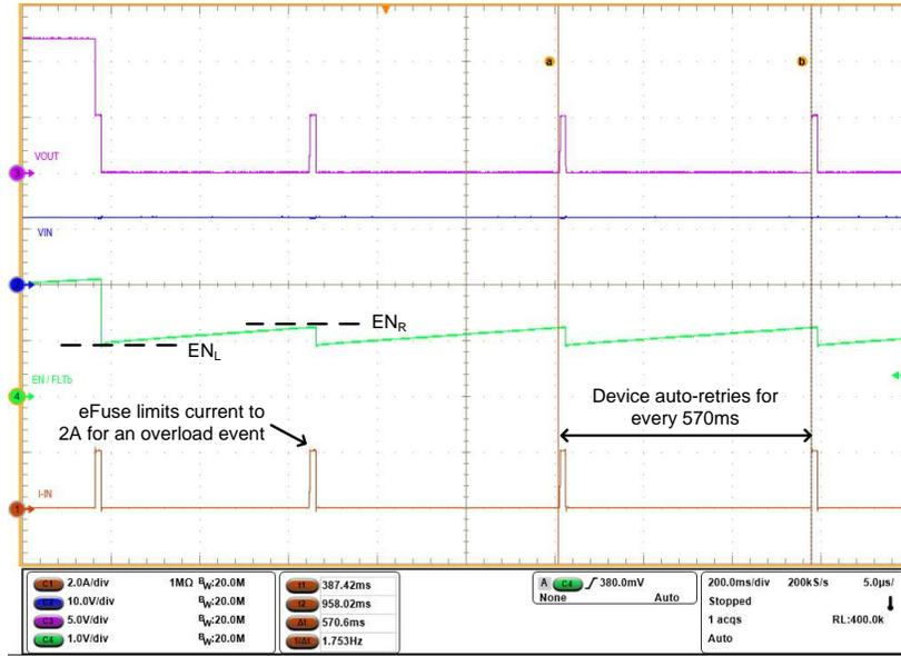
$$R_{\text{RETRY}} = 1 \text{ M}\Omega$$
