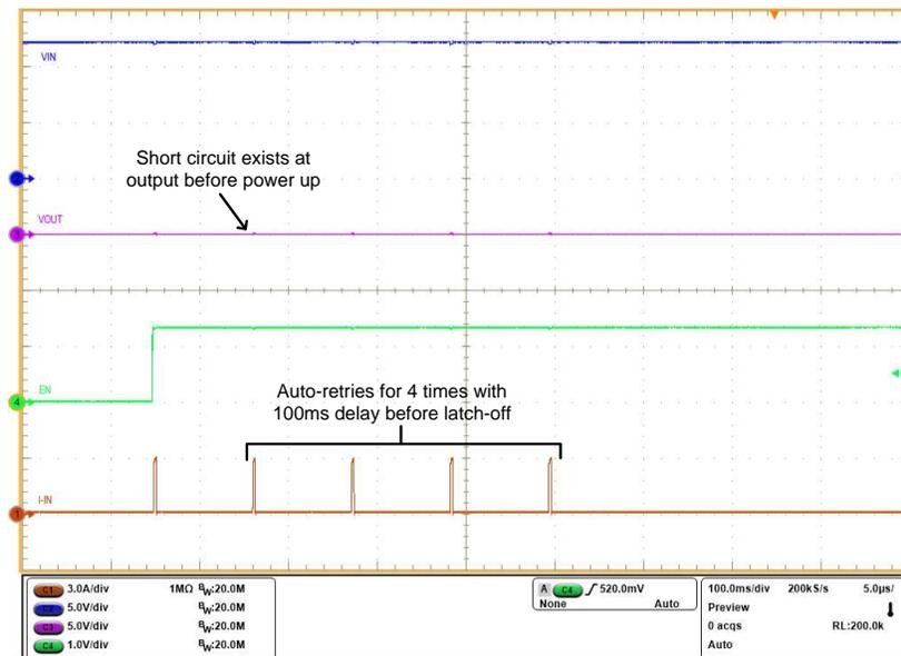
$R_{ILIM} = 332 \Omega$        $C_{TIMER} = 4.7 \text{ nF}$        $C_{RETRY\_DLY} = 2.2 \text{ nF}$        $C_{NRETRY} = 2.2 \text{ nF}$
