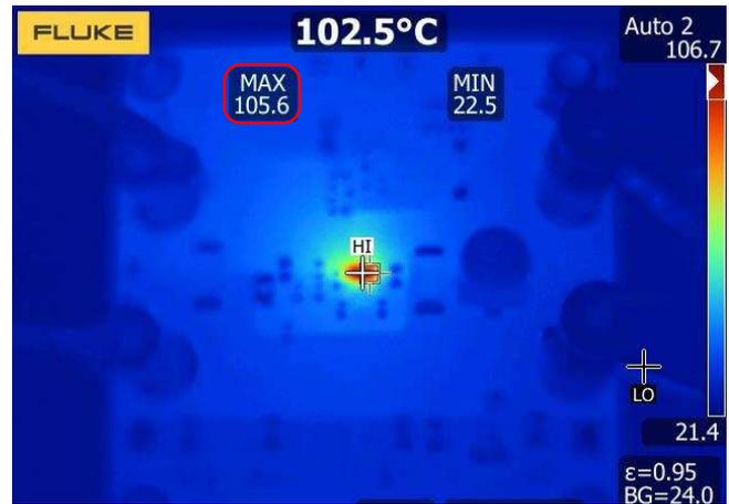
Figure 17. Case Temperature of the TPS25982 Device Under Sustained Fault with 100 ms Retry Delay
