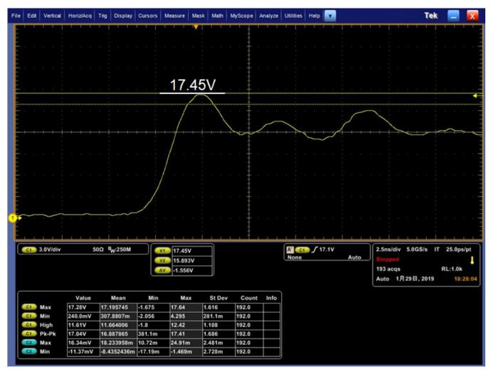
Figure 5. On-Board Test High-Side FET VDS Waveform
