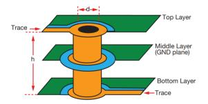
Figure 2. Parasitic Inductance of the PCB Via
