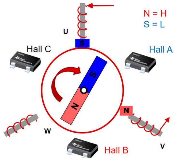
**Figure 1. BLDC Motor Model, Commutation Step 1**
