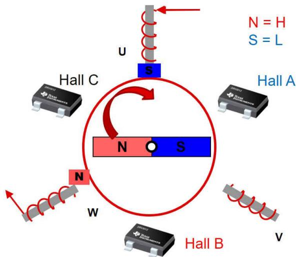
**Figure 2. BLDC Motor Model, Commutation Step 2**
