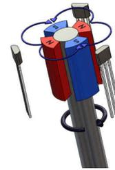
**Figure 6. Rotor Position Using TO-92 Hall Sensor**
