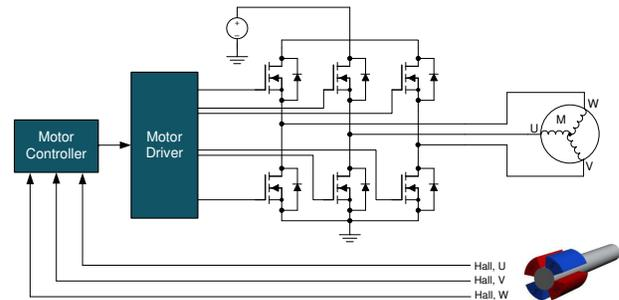
**Figure 5. Closed-Loop System for BLDC Motor Control**
