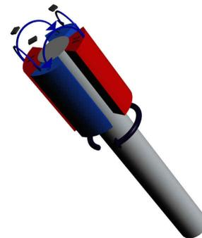
**Figure 7. Rotor Position Using Surface Mount Hall Sensor**
