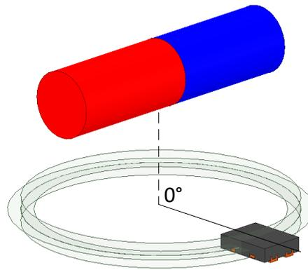
**Figure 15. Three Position Rotary Switch OFF Position**
