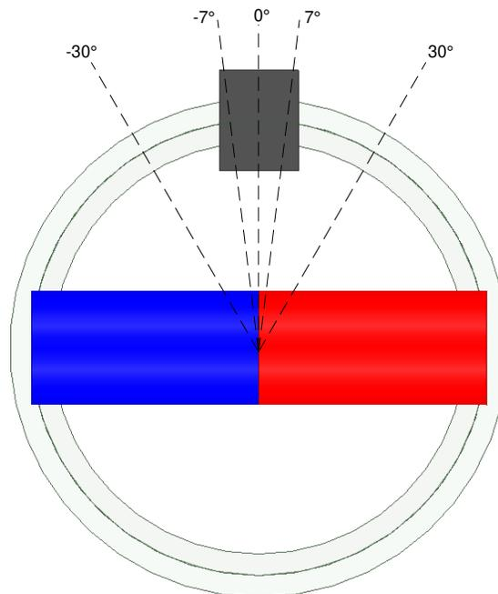
**Figure 16. Rotary Magnetic Travel for Three-Position Switch**
