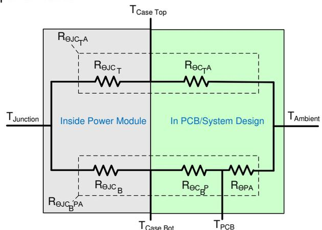
Figure 2. Thermal Resistance from Junction to Ambient
