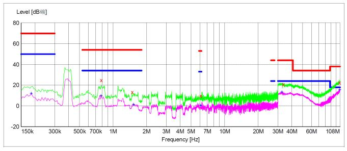
Figure 5. EMC Construction Test Result of Common TPS2583X PCB Layout
