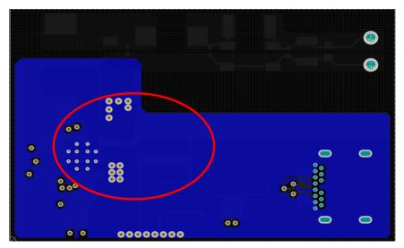
Figure 12. Bottom Layer of the PCB Layout for the TPS2583X
