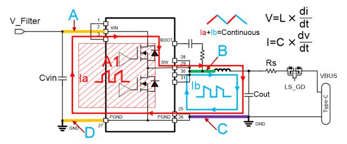
Figure 7. Buck Converter Schematic
