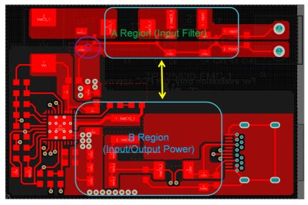
Figure 6. Single-Sided Device Placement, Multi-Layer PCB Layout
