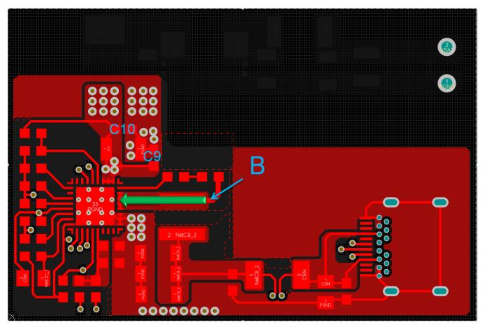
Figure 16. PCB Layout for the Power Part in the Top Layer
