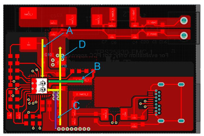
Figure 9. Power Loop of the PCB Layout for the TPS2583X
