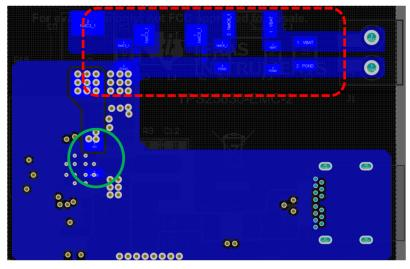
Figure 15. Bottom Layer of the PCB Layout for Input Filter
