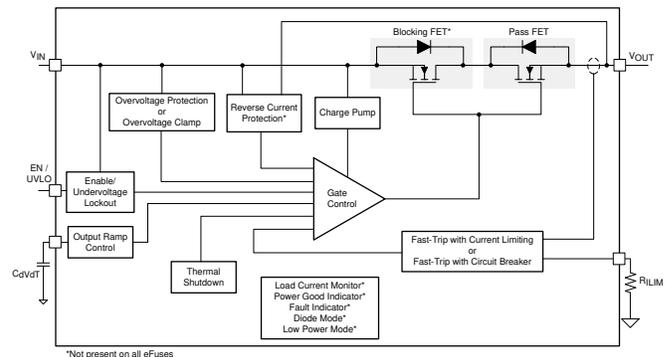
Figure 2. Simplified eFuse Block Diagram
