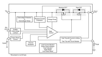
Figure 2. Simplified eFuse Block Diagram
