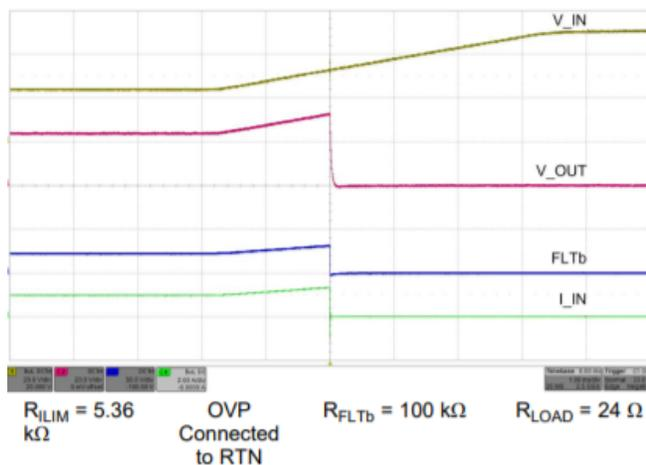
**Figure 4. TPS26600 Over Voltage Cut-off Response**
