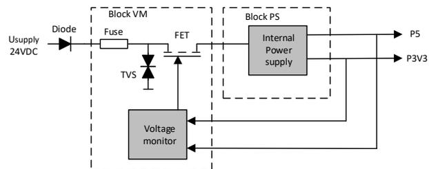
**Figure 2. Functional Blocks of Subsystem PS/VM IEC 61800-5-2 Annex A**
