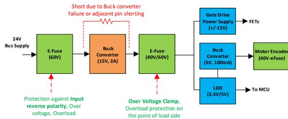
**Figure 3. Single Point Failure Protection for Buck Converter**
