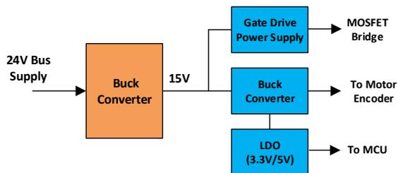
**Figure 1. Typical Block Diagram of Motor Drive Control Card Power Supply**
